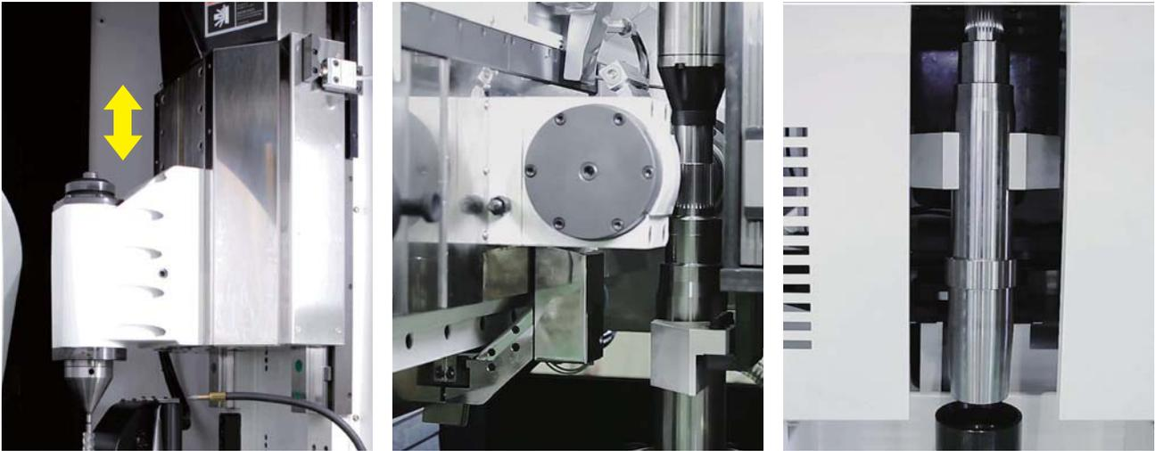
▶ It is designed to adjust tailstock position for long shaft cutting and up to 650mm shaft can be automated using ring loader
