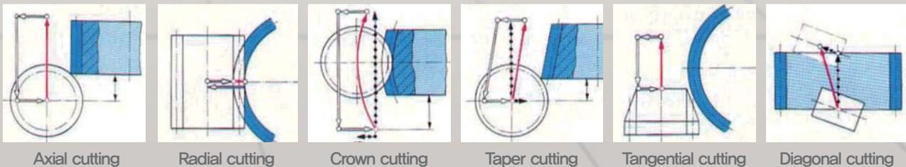
▶ This machine can use not only crown gears and taper gears, but also all hobbing cycles applied to gear cutting (axial cutting, radial cutting, tangential cutting and diagonal cutting)
