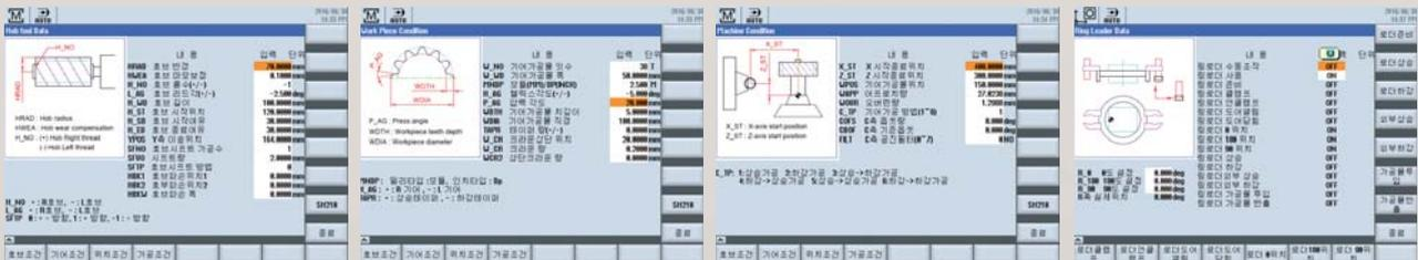
▶ By utilizing the Easy dialogue programming environment, additional programming is not necessary and gear processing is easy with just the input of specifications of hob cutter, workpiece, and cutting condition
